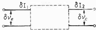
Fig. 4. Four-pole-parameter representation of transistor. Here measurable quantities are labelled generally 1 (input) and 2 (output) and replaced by notation appropriate to mode of connection. For instance, mode: common base, then 1 becomes e and 2 becomes c.
