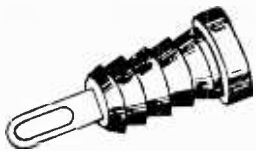
Quick-fixing chassis socket—the Fasfit—by Spear Engineering. The socket is simply pushed into place and is held by the moulded serrations.
